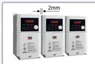
Side-by-side Installation (2mm between drives)
